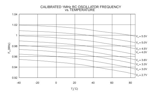
**Figure 196.** RC Oscillator Frequency vs. Operating Voltage (the devices are calibrated to 1 MHz at Vcc = 5V, T=25c)
