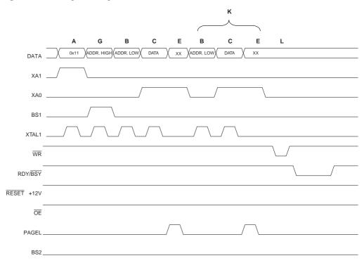
Figure 138. Programming the EEPROM Waveforms
