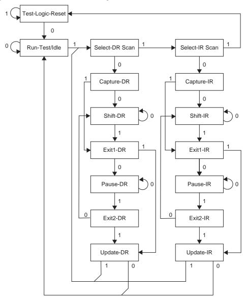
Figure 121. TAP Controller State Diagram
