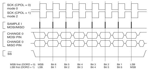
Figure 78. SPI Transfer Format with CPHA = 1
