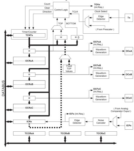
Figure 46. 16-bit Timer/Counter Block Diagram
