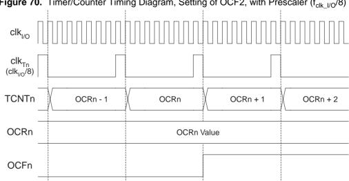
Figure 70. Timer/Counter Timing Diagram, Setting of OCF2, with Prescaler ( $f_{clk\_l/O}/8$ )
