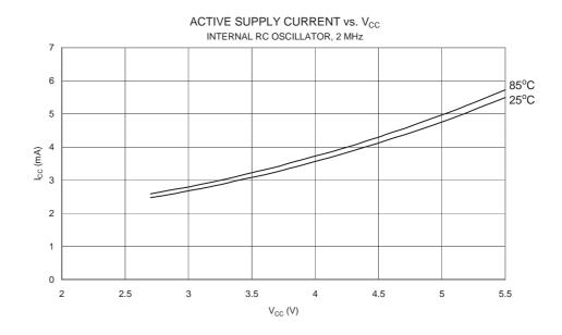
Figure 163. Avtive Supply Current vs.  $V_{CC}$ , Internal RC Oscillator 4 MHz
