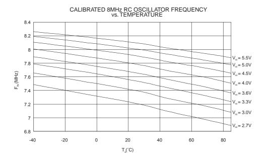
**Figure 202.** RC Oscillator Frequency vs. Operating Voltage (the devices are calibrated to 8 MHz at Vcc = 5V, T=25c)
