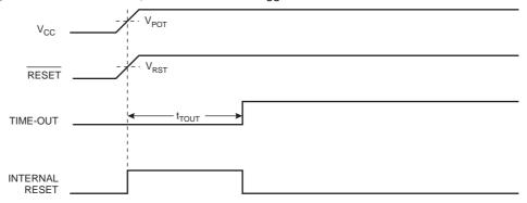
Figure 24. MCU Start-up, RESET Extended Externally
