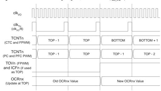
Figure 58. Timer/Counter Timing Diagram, with Prescaler (fclk 1/0/8)
