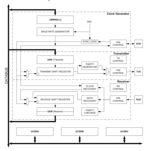
Figure 79. USART Block Diagram
