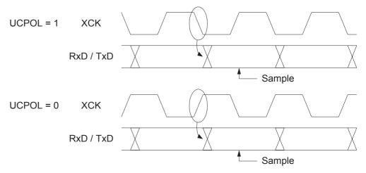
The UCPOL bit UCRSC selects which XCK clock edge is used for data sampling and which is used for data change. As Figure 81 shows, when UCPOL is zero the data will be changed at rising XCK edge and sampled at falling XCK edge. If UCPOL is set, the data will be changed at falling XCK edge and sampled at rising XCK edge.
