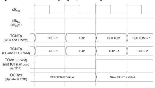
Figure 58 shows the same timing data, but with the prescaler enabled.
