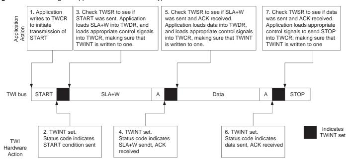
The first step in a TWI transmission is to transmit a START condition. This is
