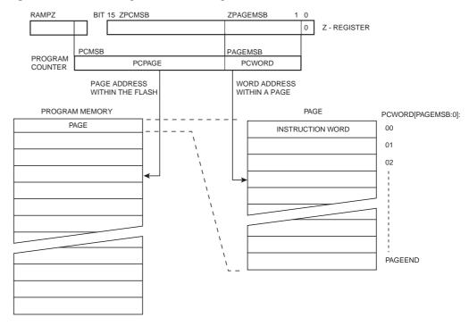
Note: 1. The different variables used in Figure 134 are listed in Table 115 on page 284.
