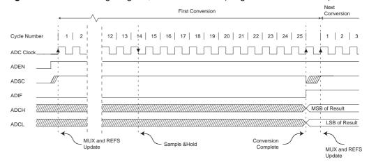
Figure 111. ADC Timing Diagram, Single Conversion
