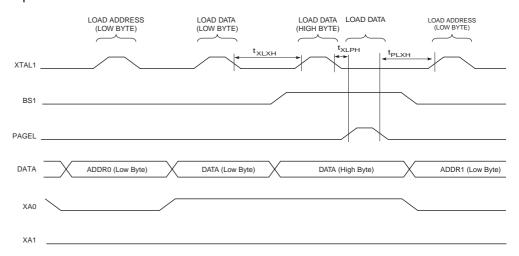
Note: The timing requirements shown in Figure 141 (i.e.  $t_{DVXH}$ ,  $t_{XHXL}$ , and  $t_{XLDX}$ ) also apply to loading operation.
