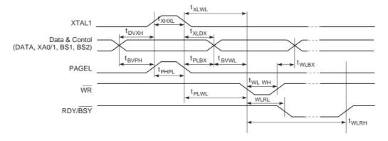
**Figure 142.** Parallel Programming Timing, Loading Sequence with Timing Requirements
