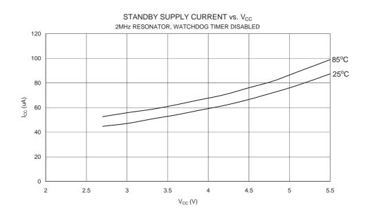
Figure 177. Standby Supply Current vs. V<sub>CC</sub>, 2 MHz Xtal, Watchdog Timer Disabled
