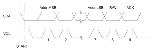
Figure 89. Address Packet Format
