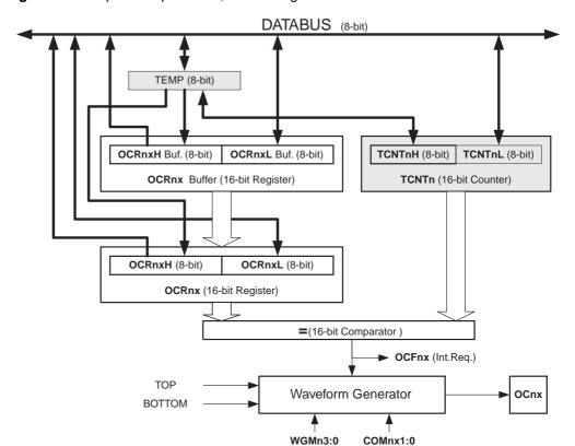
Figure 49. Output Compare Unit, Block Diagram
