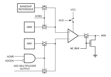
Figure 130. General Boundary-scan Cell used for Signals for Comparator and ADC
