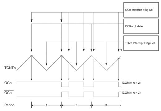
The Timer/Counter Overflow Flag (TOV2) is set each time the counter reaches BOTTOM. The interrupt flag can be used to generate an interrupt each time the counter reaches the BOTTOM value.
