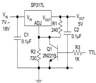
Figure 15. 5V Logic Regulator with Electronic Shutdown (Minimum output = 1.2V)
