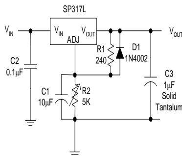
Figure 18. Adjustable Regulator with Improved Ripple Rejection
