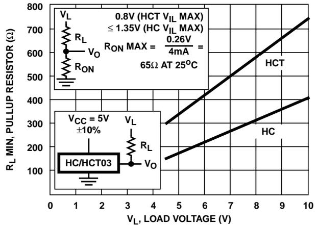
**FIGURE 2. MINIMUM RESISTIVE LOAD vs LOAD VOLTAGE**
