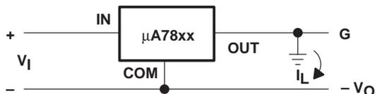
**Figure 2. Positive Regulator in Negative Configuration (V<sub>I</sub> Must Float)**
