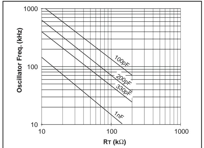
Figure 4. UCC1800/1/2/4 oscillator frequency vs.  $R_T$  and  $C_T$ .
