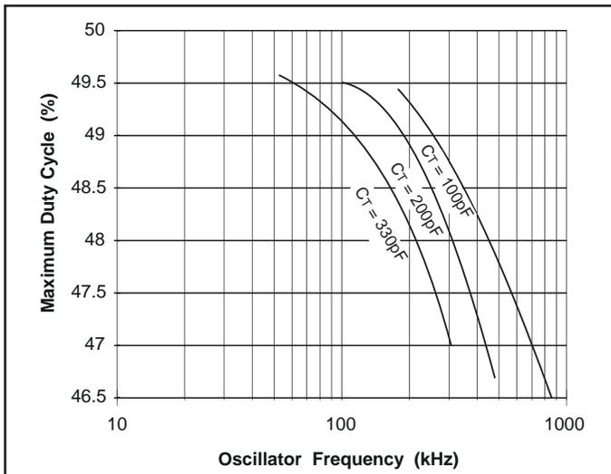
Figure 7. UCC1801/4/5 maximum duty cycle vs. oscillator frequency.
