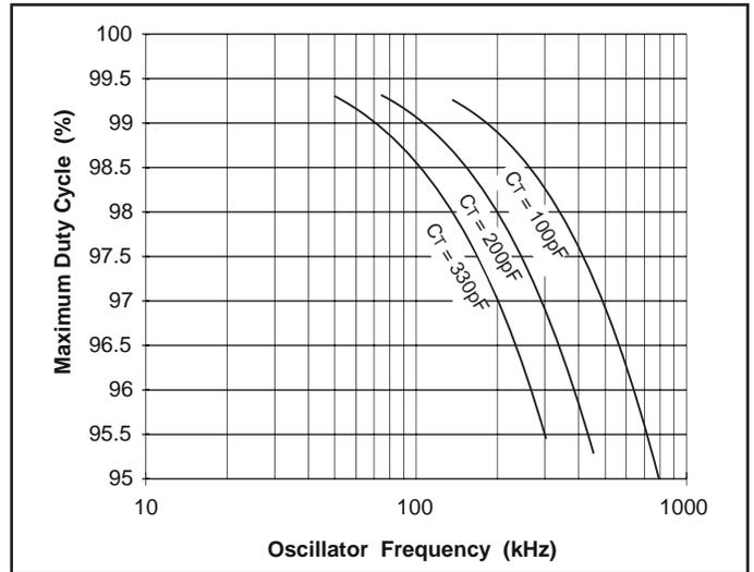
Figure 6. UCC1800/2/3 maximum duty cycle vs. oscillator frequency.
