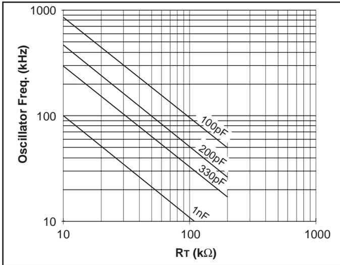
Figure 5. UCC1803/5 oscillator frequency vs.  $R_T$  and  $C_T$ .
