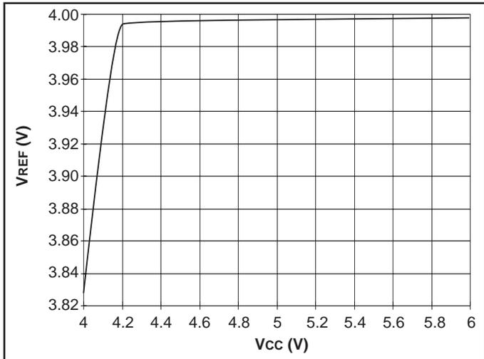
Figure 3. UCC1803/5  $V_{REF}$  vs.  $V_{CC}$ ;  $I_{LOAD} = 0.5mA$ .
