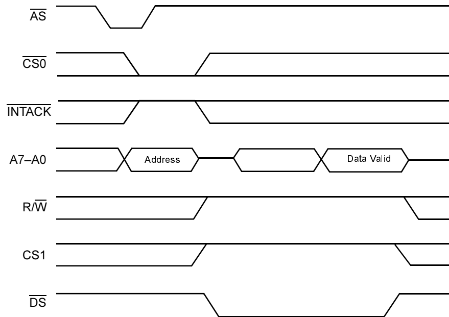
Figure 19. Z80230 Read Cycle Timing
