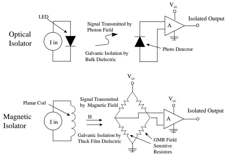
Figure 2. Analogy between GMR isolator and conventional opto-isolator
