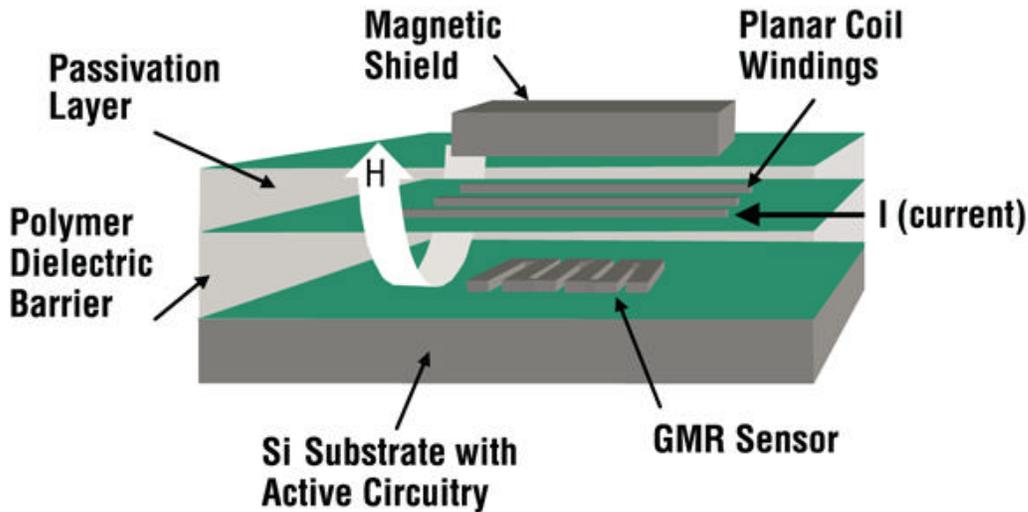
Figure 1. GMR Galvanic Signal Isolator Concept
