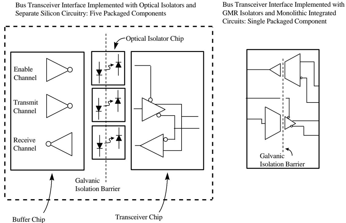
**Figure 3: Example of Combined Horizontal and Vertical Integration**
