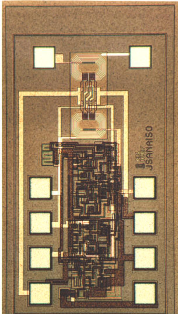
**Figure 4: Photomicrograph of Isolated Linear Amplifier**
