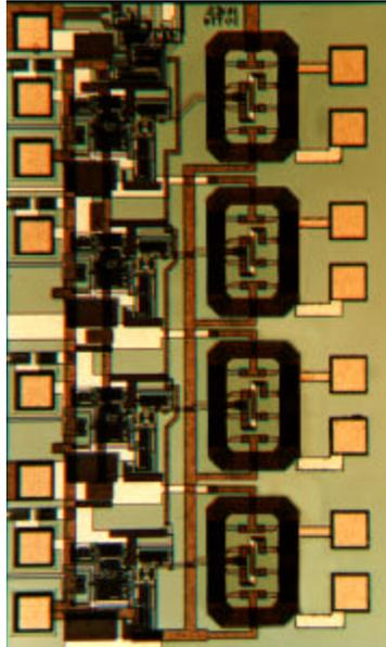
**Figure 5: Four Channel Isolated Receiver Die**
